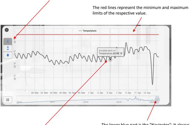
If you touch the line at a specific point, detailed information about the measurement data at that point is displayed. The lower blue part is the "Navigator": It always shows the complete history of the measured data. The Navigator limits the area that you can see at the top of the diagram. You can move, zoom in and out of the Navigator as you wish, which also changes the data displayed.
